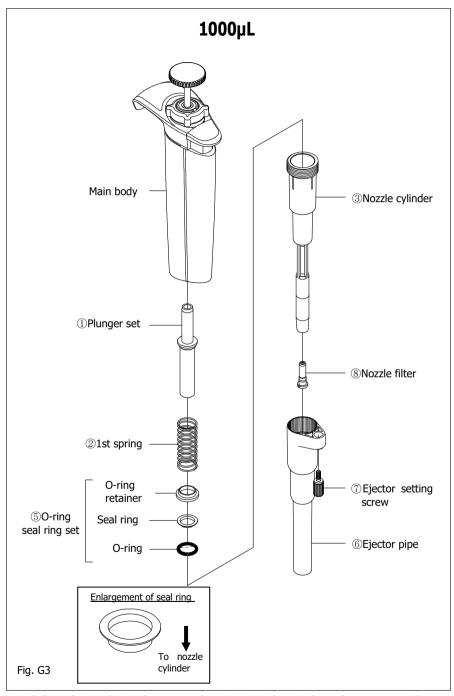
Circled Numbers in (Fig. G3) corresponds to Parts Numbers in the replacement parts list.
