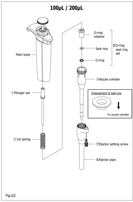
Circled Numbers in (Fig. G2) corresponds to Parts Numbers in the replacement parts list.
