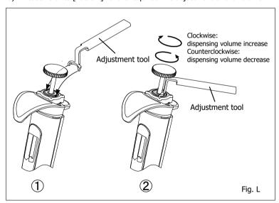
Circled Numbers in (Fig. L) corresponds to Parts Numbers in the replacement parts list.
