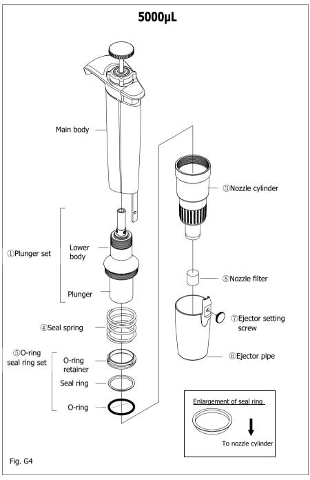
Circled Numbers in (Fig. G4) corresponds to Parts Numbers in the replacement parts list.
