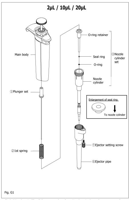
Circled Numbers in (Fig. G1) corresponds to Parts Numbers in the replacement parts list.
